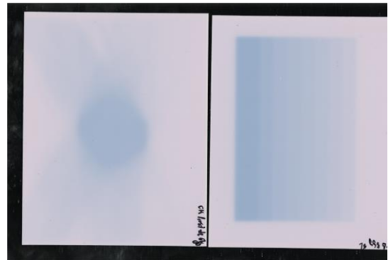
Figure 4: Exposed OC-1 Film scanned from left to right, Calibration field (right), Treatment Field (left)
